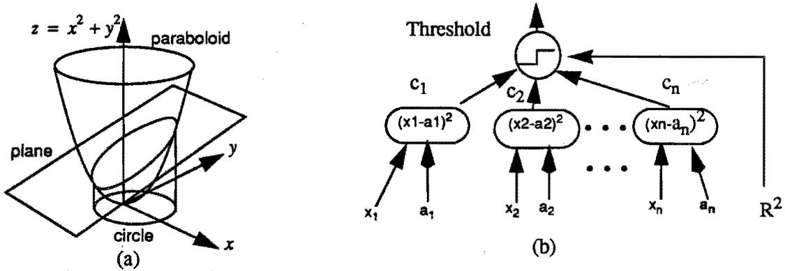
Figure 2 (a) The plane intersects the paraboloid in a curve which projects to a circle. (b) Architecture of threshold unit computing the intersection in  $n$  dimensions.
