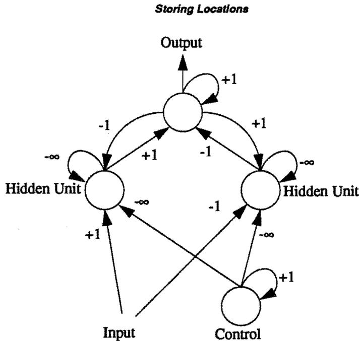
Figure 4 Schematic of a binding network. The network continually tracks its input signal until a control signal is sent, at which point the output is frozen to be the current signal.
