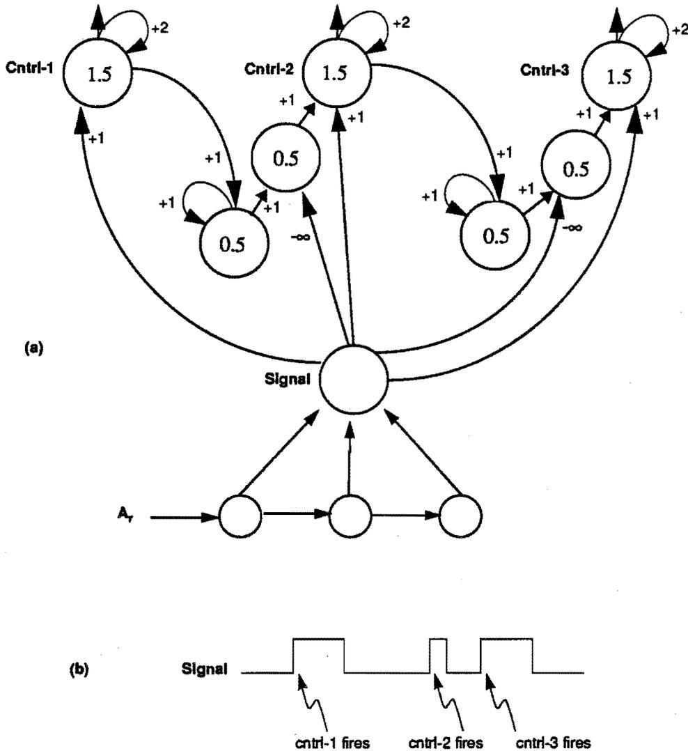
Figure 6 A detailed diagram of a portion of the sequencer. The units shown above sends control signals to the appropriate binding networks. The signal unit fires when all of its inputs are equal. The first time it fires, cntrl-1 starts firing. The next time, cntrl-2 fires, and so on. This structure is used to send control signals to successive binding networks.
