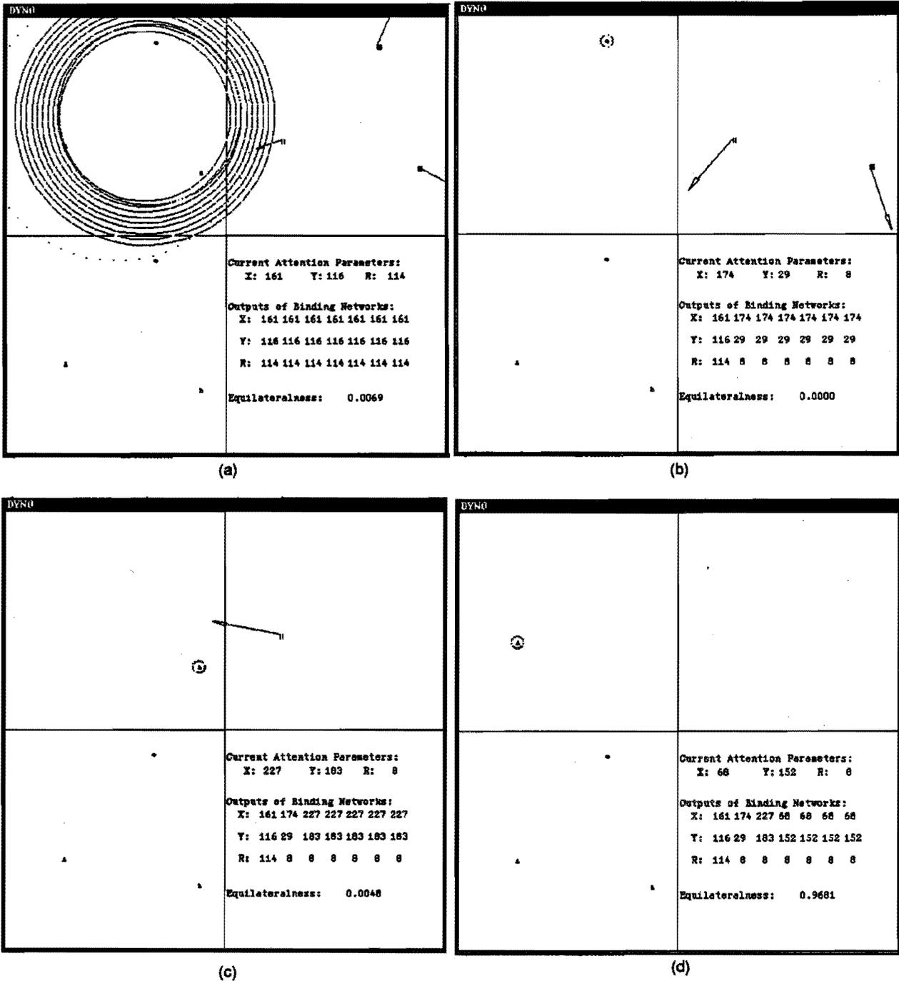
Figure 6 Four steps in a typical run. (a) Determining the size and location of the whole triangle. (b) - (d) Network after fixating on each of the three vertices. Note that the binding networks are updated correctly. Once all four positions are available, the network correctly classifies the triangle to be equilateral (bottom right of (d)).
