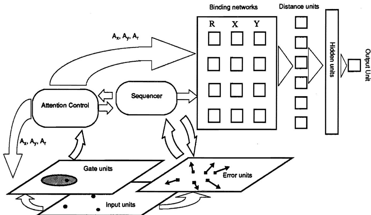
Figure 5 Basic system architecture. The module "Attention Control" continually tries to fit the focus of attention to the points within it. The "Sequencer" updates the focus of attention to visit all the clusters in sequence and also sends the control signals to the binding network to store successive locations.
